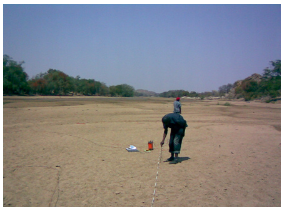
MSc student carrying out geophysical research. At the Malala site, MSc student Taurai Masvopo carried out tens of resistivity surveys to establish the depth of the sand.
