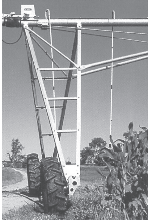
FIGURE 10.5 - The Support towers.
