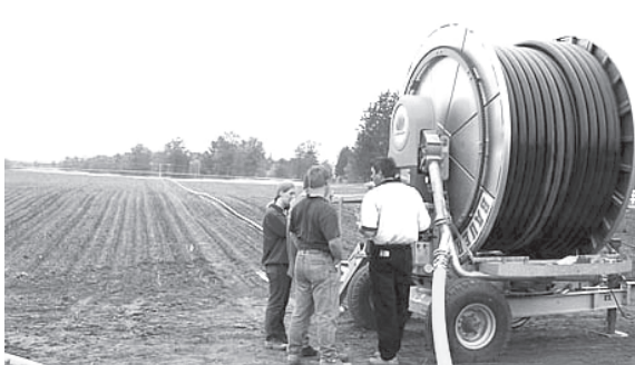
FIGURE 9.4 - The reel machine with the PE pipe.
