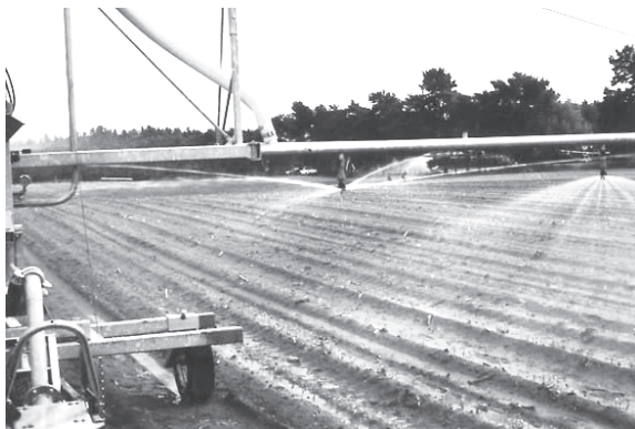
FIGURE 9.3 - The full-circle and the half-circle Sprayers.
