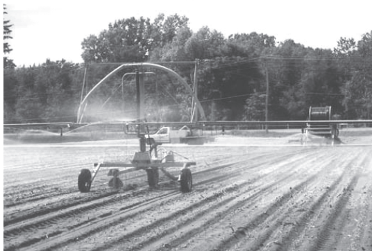
FIGURE 9.2 - The boom, the PR pipe and the reel machine.
