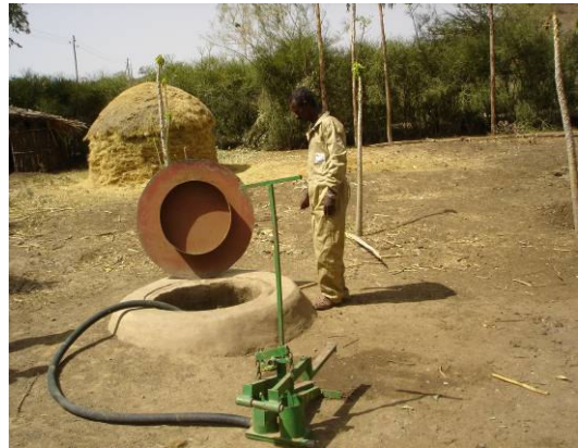
Figure 6: The treadle pump used by farmers
