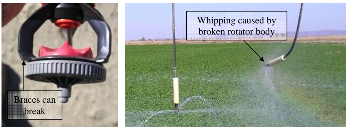
Figure 10. Non-functioning sprinkler because of broken rotator body
