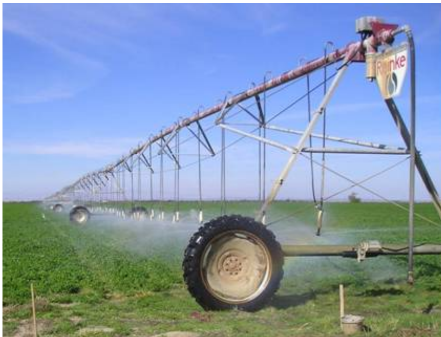
Figure 4. Original sprinkler heights – average 3.5 feet
