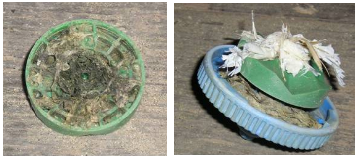
Figure 8. Sprinklers with trash on rotator plates
