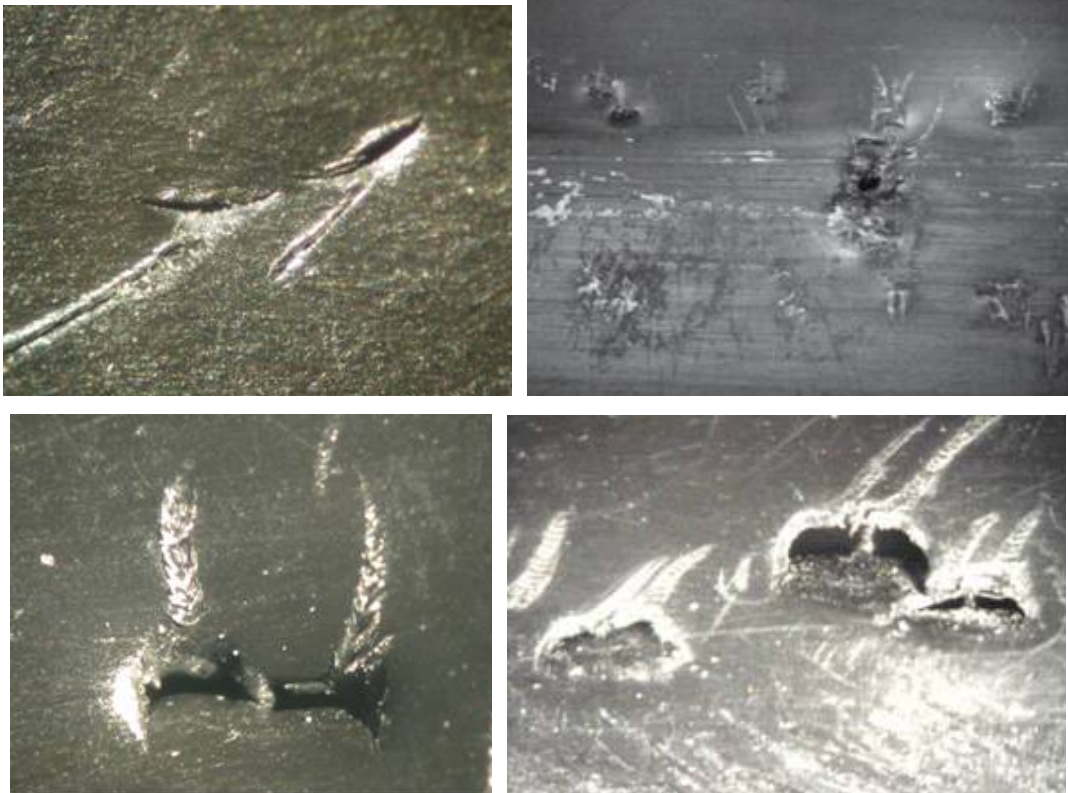
Figure 7. Examples of rodent damage, generally with characteristic scratch marks.
