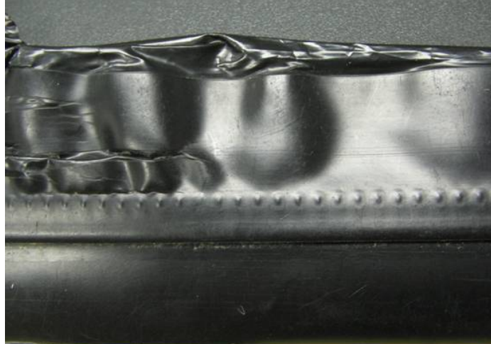
Figure 21. Tape damage due to excessive pressure
