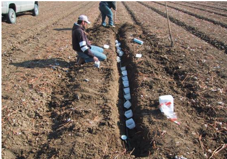
Figure 2. Freezerettes lined up in preparation for flow measurement of individual emitters. Notice the pressure gauge in the foreground.
