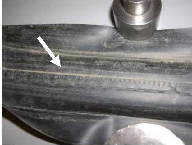
Figure 16. Plugged inlets to the emitter path
