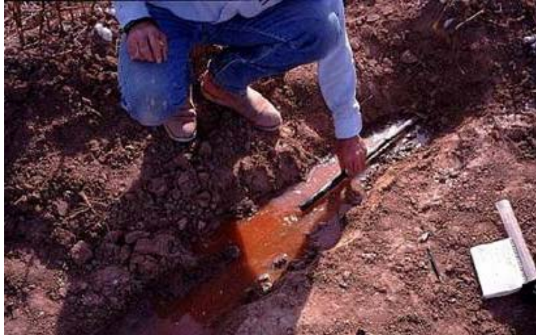
Figure 19. Chemical precipitate flushed from tape. The unidentified chemical compound was supposed to be a fertilizer. It was injected downstream of the filters and plugged a complete irrigation system.
