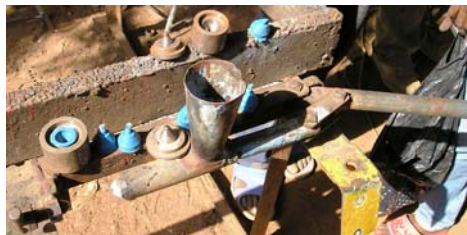
PE piston mould and extruder
