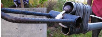
guide box with rope and pistons running through.
