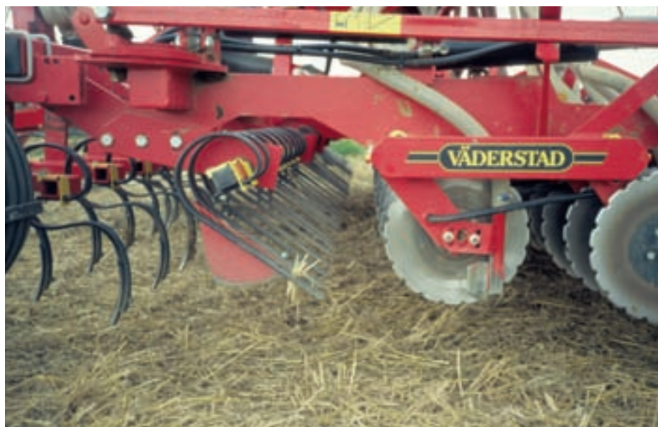
Detailed view of the 'Väderstad Rapid Cultivation Drill' with tines and discs. (Alastair Leake)
