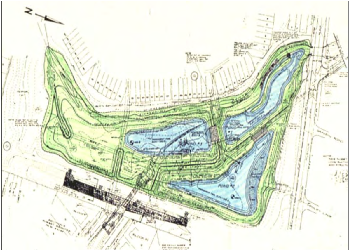
Figure 7: Conflict with a major sewer was avoided by using a berm and a three cell design in this retrofit.
