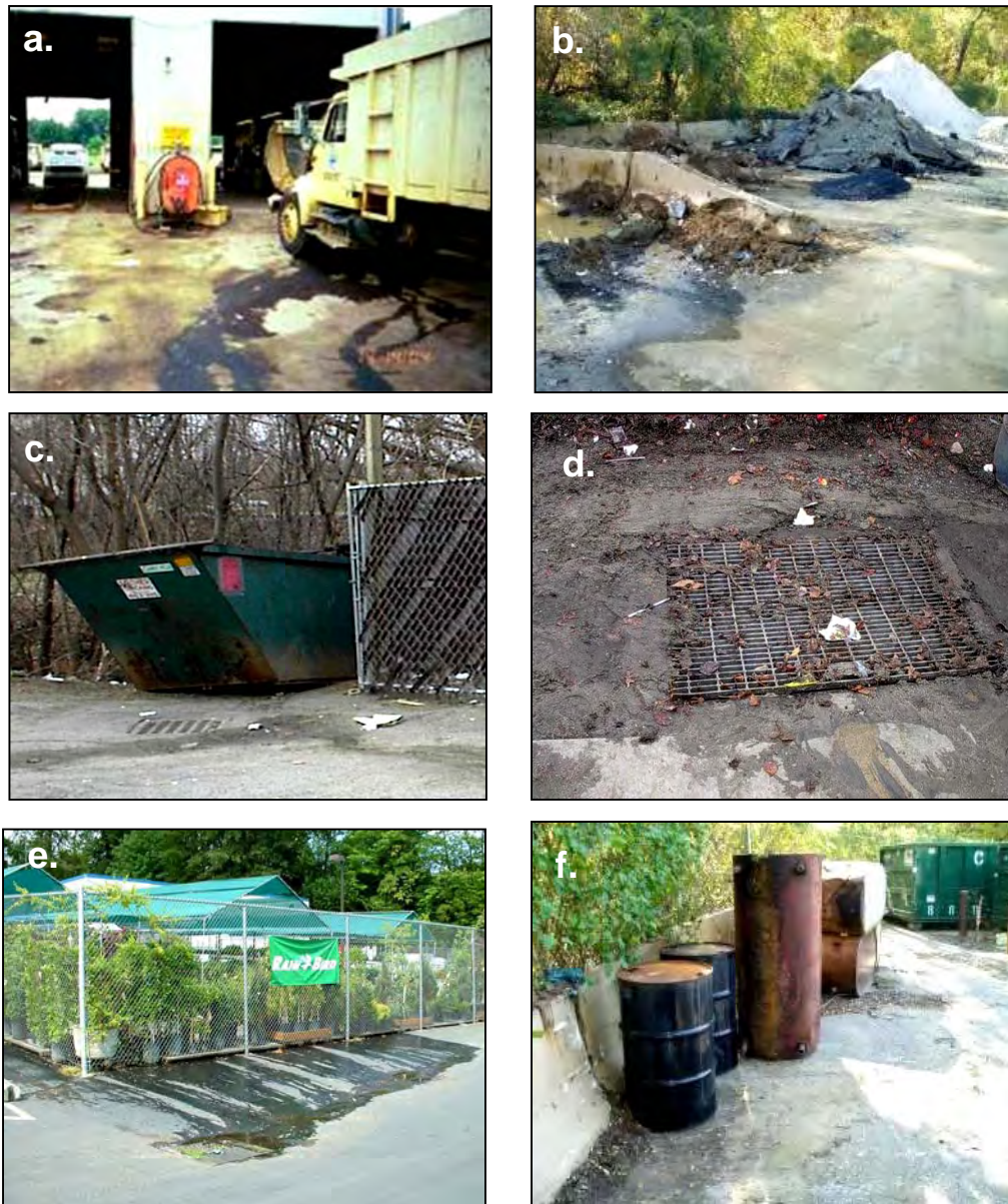
Figure 4: Common hotspot generating areas to look for during a site investigation: vehicle service/fueling (a); bulk outdoor storage(b); dumpsters (c); truck washouts (d) irrigation/fertilization (e); and chemical drums (f).
