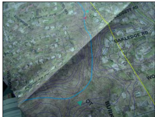
Figure 4.2: This sample base map includes aerial photography, 5-foot contours, hydrology, and locations of sites to be assessed.
