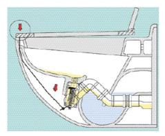
Figure 8. Schematic showing the valve on the urine pipe to collect urine without flushing water in the Roediger "NoMix toilet" – valve opens when the user is seated (source: Roediger).
