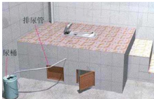
EcoSan toilet pedestal and squatting pan in Guanxi, China (source: gtz, 2005)
