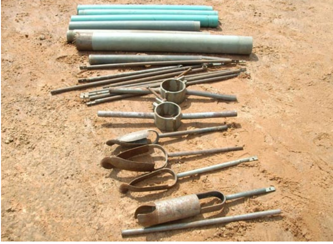
Figure 9 Augers, Bailers, Clamps and Casings
