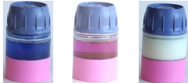
B2P water testing kit. (blue: no coliforms in sample, pink: presence of coliforms, white: presence of E.coli)
