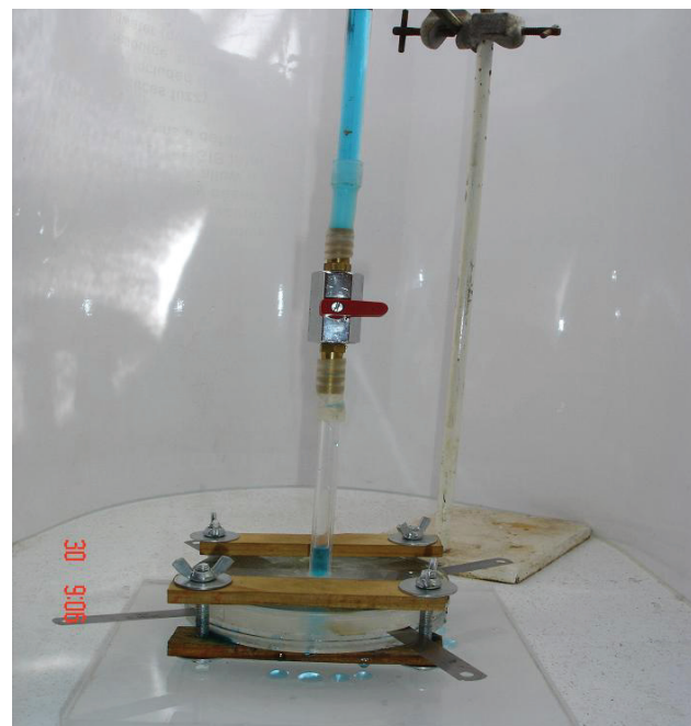
Figure 6 Laboratory apparatus for the fracture aperture determination experiment using blue-coloured water. Note the clamped thickness gauge blades to create the fracture aperture between 2 circular 100 mm diameter Perspex plates.
