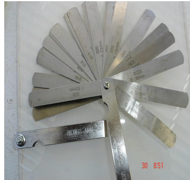
Figure 5 Thickness (feeler) gauge with the thickness of the blades printed on it. The blades are clamped between Perspex sheets to create fractures whose apertures have corresponding values.
